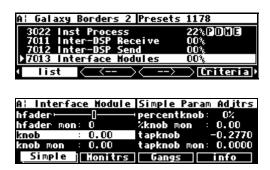
With the cursor highlighting knob on the INPUTS menu page in the LEVELS area, press and hold the SELECT key until the EXTERNAL MODULATION menu page below displays. This routine is how you can control remotely any parameter in the H7600.
